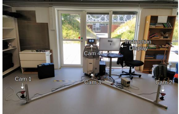
Figure 4: Recording setup. A display instructs the subject which gesture to perform to the robot. This is recorded with four different cameras.
