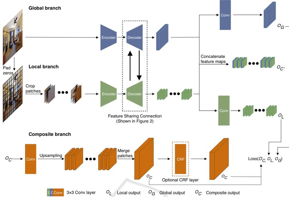
Figure 1: **CAM-SegNet** architecture. The feature maps in the decoders are shared between the global and local branches. After the encoder-decoder component, the feature maps at the same spatial location are concatenated together and passed into the composite branch, which upsamples the feature maps to the same size as the original input image. The composite output can be refined by an optional CRF layer.
