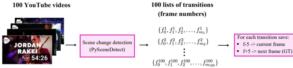
Figure 4: Extraction of the current frame and ground truth in the process of generating our data set.
