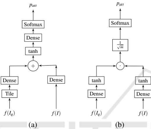
Figure 3: Computation graph of the attention mechanism  $f_{Att}$  for additive (a) and scaled dot-product (b) attention.
