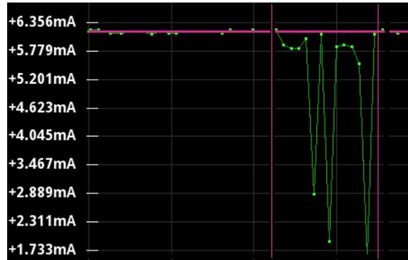
Figure 9: Current consumption of the transmitting state.
