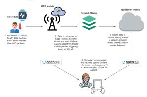
Figure 3: System Component Connection.
