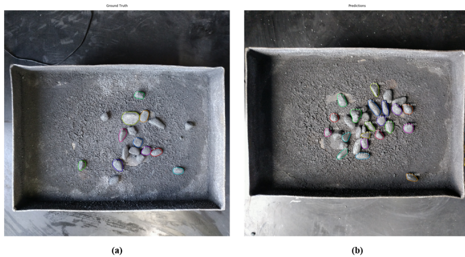
Figure 3: An example image of particles of class ‘8-9’ from training 4. In a) the highlighted particles as particles labeled and calculated as ground truth, and in b) the highlighted particles represent the particles found by the model in the prediction.
