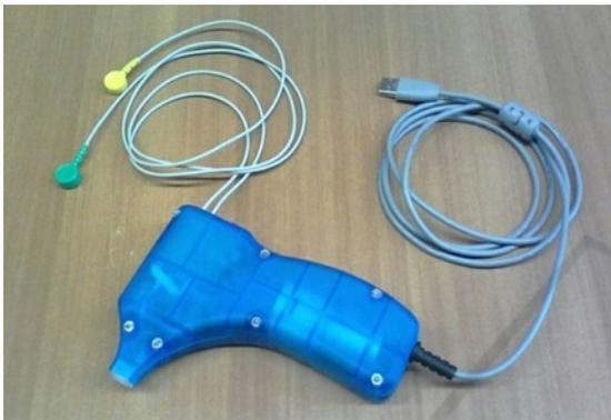
Figure 2: The version of the pressure sensor for measuring short patterns of blood pressure with a built-in ECG channel (two coloured button connectors).
