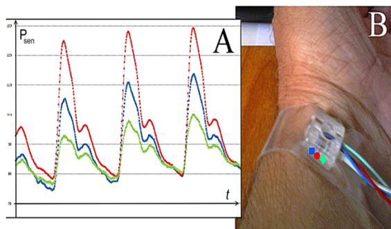
Figure 1: Three-channel pneumatic sensor for continuous non-invasive arterial blood pressure monitoring (B). The difference is the shape of the pulse wave signal from the sensor (A), depending on the position of the sensor pads: ● – pad is directly over the artery, ■, ◆ – pad is shifted to the left and to the right respectively from the central projection of the radial artery.
