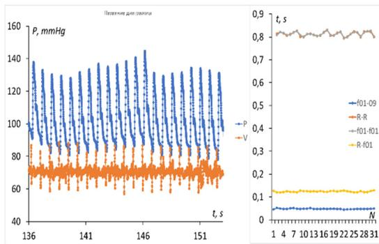
Figure 8: Pulse wave and ECG recording and their temporal characteristics for the radial artery (point 3).
