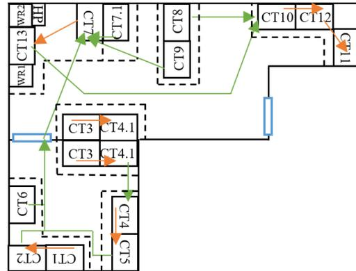
Figure 6: ICP production line layout resulting from the SLP approach.
