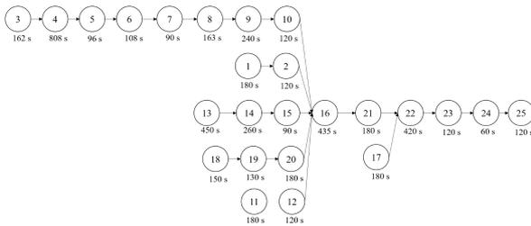
Figure 2: ICP precedence diagram.
