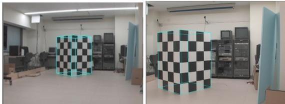
Figure 8: Left: Calibration result at reference pose, Right: Calibration result after pan / zoom.
