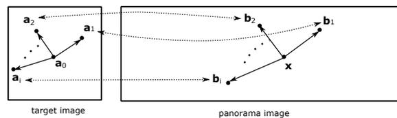
Figure 6: The left figure denotes a cylindrical image transformed from the perspective image. The right figure denotes the panoramic image of the background.
