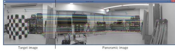
Figure 9: The left end is the image of the target taken after pan-zooming the camera. The right part is a panoramic image of the background. The result of matching both by AKAZE (Alcantarilla et al., 2013) is shown by straight lines connecting the corresponding feature points.
