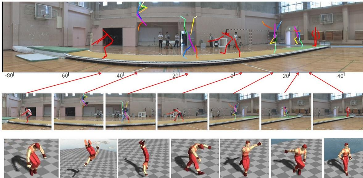
Figure 10: Upper row: The sampled results of motion capture are overlapped on the panoramic images as a stick model. Middle row: Arrange sampled tracking results which match the panoramic image at position indicated by red arrow. Lower row: Corresponding CG images of the athlete reconstructed from different camera view.
