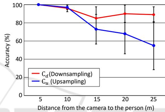
Figure 4: Accuracy of person re-identification when changing the camera–person distance.
