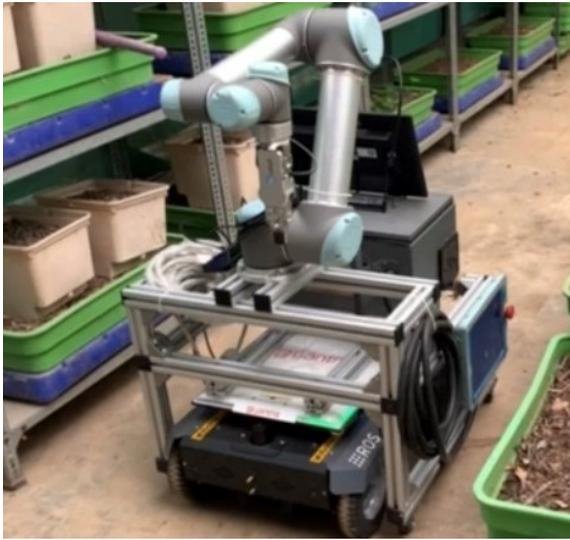
Figure 1: Custom AMAR housing few sensors with limited hardware capability.
