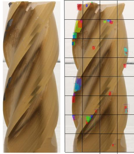
Figure 5: Results of a high-resolution damage detection and instance segmentation of an TiN coated milling tool. On the right the damages are marked with the bounding boxes and the prediction probability.
