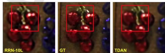
Figure 2: Example of upscaled images that vary in detail-restoration quality. The rightmost image is visually more natural, but the shape of the details in the leftmost image is closer to the original.
