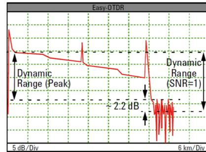
Figure 3: Dynamic range definitions with two definitions of the noise floor.
