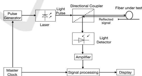
Figure 1: OTDR architecture.
