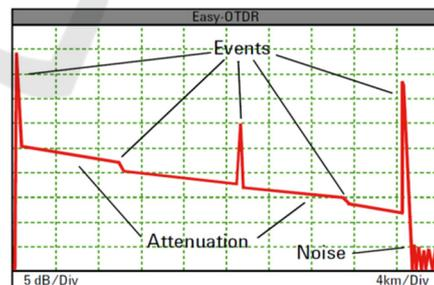
Figure 2: Typical OTDR trace for a longer fiber with various reflective and refractive events (5 dB/Div; 4 km/Div).
