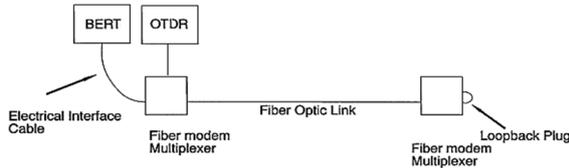
Figure 6: OTDR and two-way BERT configuration.
