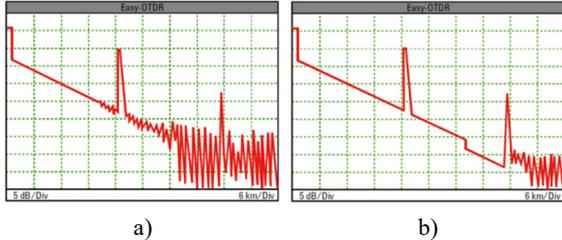
Figure 4: OTDR trace; a) small dynamic range, b) large dynamic range.
