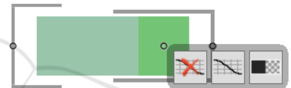
Figure 4: A context menu for editing of this Tube to change the buffer time from a continuous to a discrete one (right), add a new probability distribution (center), or remove a probability distribution (left).
