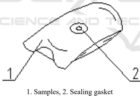
Figure 2: Schematic diagram of gas sampling with gas collection device.
