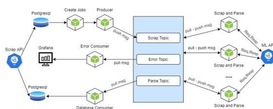
Figure 1: Architecture of the Scraping System.
