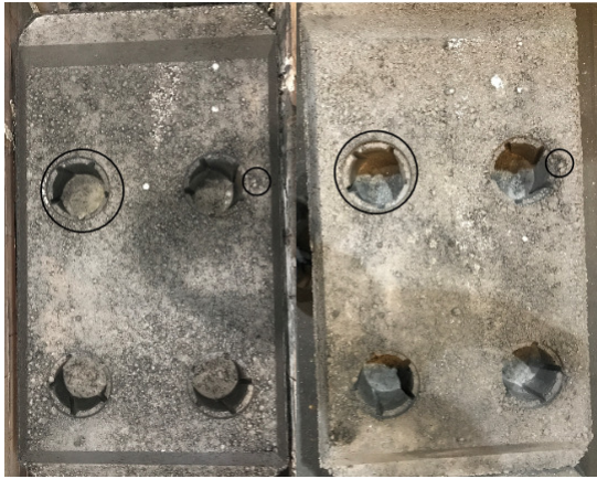
Figure 3: Variances in surface texture before (left) and after (right) the anode is baked in the furnace. Notice that the anode is lighter afterwards, which is the case at every baking.
