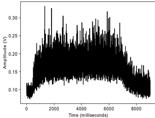
Figure 1: An Acoustic Emission Signal from Sensor mounted on the Worktable.
