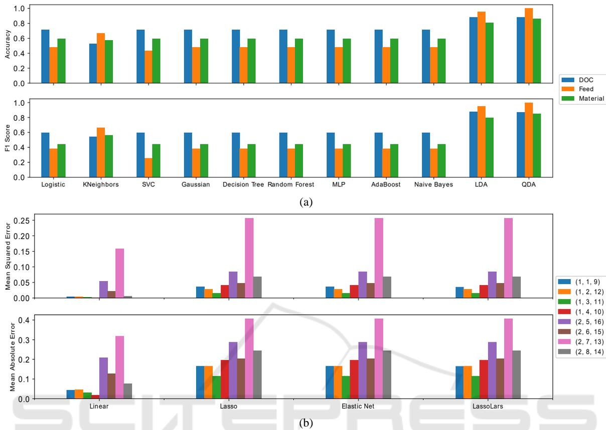
Figure 4: Model Performances (a) Classification Models: AE vs DOC, Feed, Material (b) Regression Models: AE vs Tool Wear.
