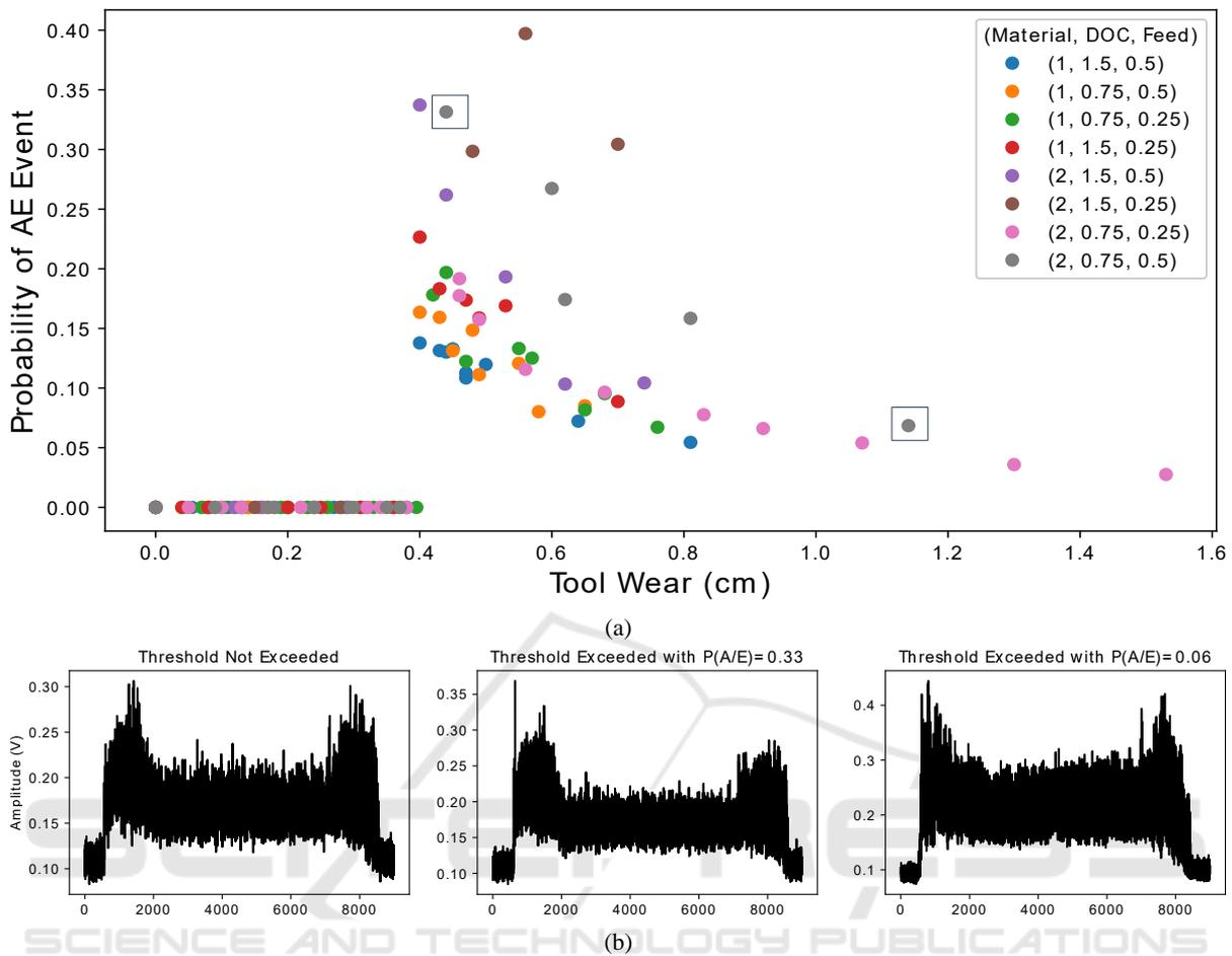
Figure 5: Comparisons of AE Events with Actual Signals (a) Progression of Tool Wear with every AE Event (b) AE Events from Cases 8 and 14.
