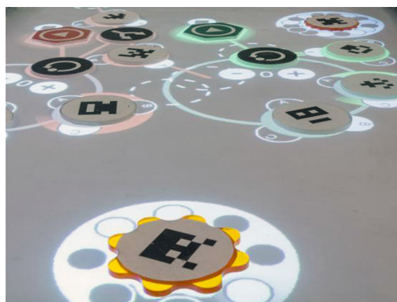
Figure 3: Fiducial markers in use in TuneTable .
