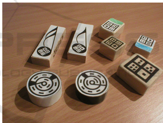
Figure 2: Fiducial markers in use in D-Touch . Picture taken from (Costanza et al., 2003).
