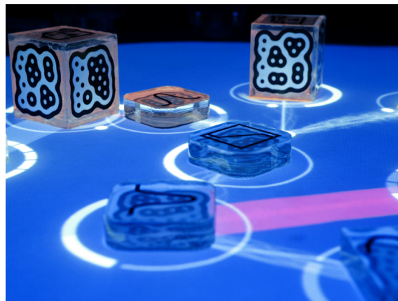
Figure 1: Fiducial markers in use in the reacTable . Picture taken from (Dance Music Northwest, 2015).
