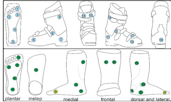
Figure 3: First line: Placement of the 17 pressure sensors of ski boot prototype 'PTBoot' (placed on the inner side of the hard shell of the boot). All sensors have a diameter of 30 mm. Second line: Placement of 17 pressure sensors in the sock prototype 'PTSock' and the placement of the sensors directly on the skin of the foot 'PTFoot'. Sensors 6, and 10 are of a smaller diameter (20 mm). All other sensors have a diameter of 30 mm.
