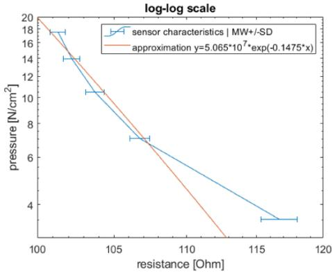
Figure 2: Sensor characteristic of the large sensor type derived of 5 of the self-made pressure sensors.
