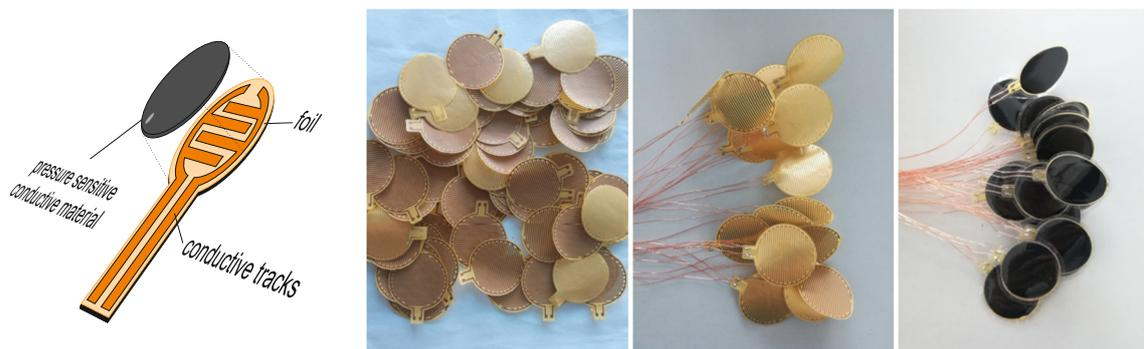
Figure 1: Schema of the pressure sensor (left) and steps of manufacturing: middle left: foils with conductive tracks; middle right: wired sensor foils; right: finished sensor with pressure sensitive conductive material layer over the foils with the conductive tracks and protective, non-conductive foils laminated on both sides of the sensor.
