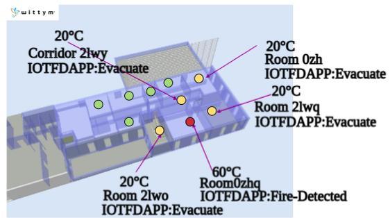
Figure 6: Result of IOTFDAPP displayed in WITTYM-BIM. The plan in 3D belongs to the rooms of our laboratory building floor.
