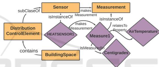
Figure 4: Part of T-Box and A-BOX from sensors and their measurements extracted from B<sup>2</sup>rainKR.
