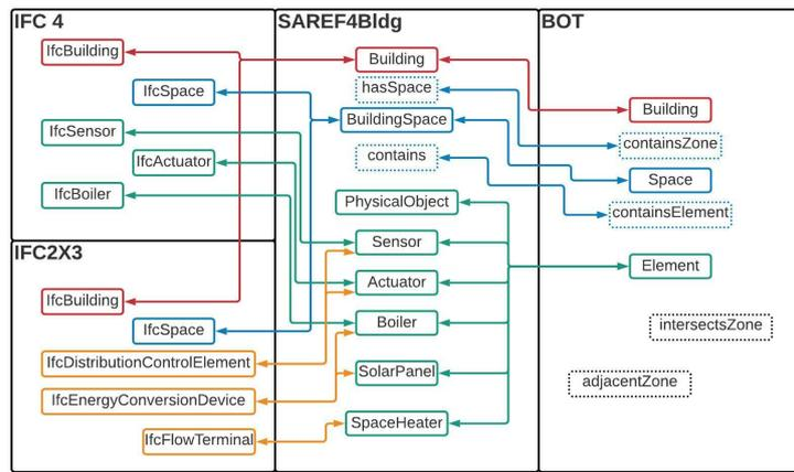
Figure 2: The windows IFC4, IFC2x3, and SAREF4Bldg represent the alignments between IFC and SAREF4Bldg concepts. The two-sense arrows indicate the equivalence, and the color code represents main concepts such as Building (red), Spaces (blue), and Objects (green). In IFC2x3 as no direct or explicit equivalence, the yellow block contains the general ancestor of IFC2x3 objects. The windows SAREF4Bldg and BOT display the alignment between them and the properties (dotted blocks).
