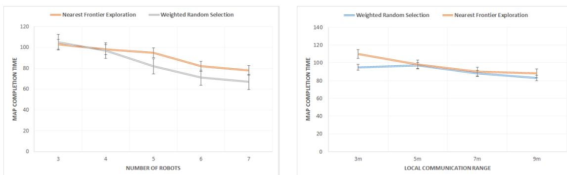
(a) The trend in exploration completion time with respect to the number of robots. (Local communication range = 5m) (b) The dependence of the algorithms to the local communication range. (For five robot fleet)
