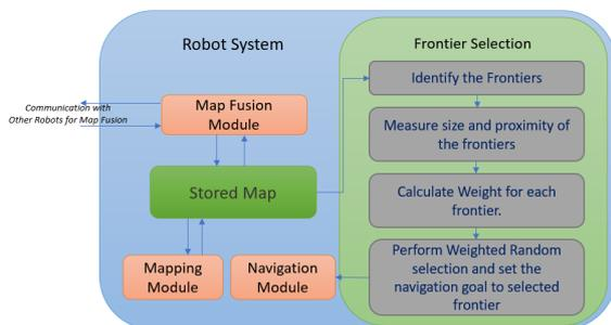
Figure 1: A schematic diagram showing the robot systems module and their interactions. Note that the communication is only required for the Map Fusion, and the frontier selection is performed within the robot system.
