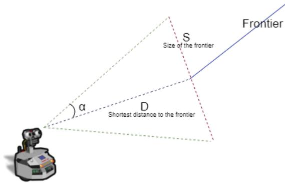
Figure 2: Diagram showing how the weight corresponds to the angle made by the frontier in robot vision.
