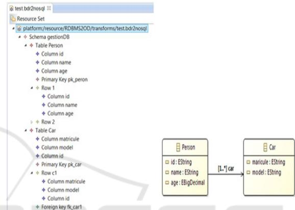
Figure 7: RDBMS source model: EMF model and instance model.
