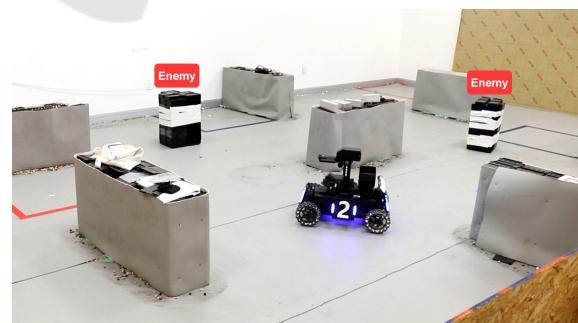
Figure 1: The arena used for experiments. As enemies don't change position during iterations, we use two plastic boxes (in black, at the figure) to emulate their positioning, forcing our robots to use LiDAR sensors to localize them.
