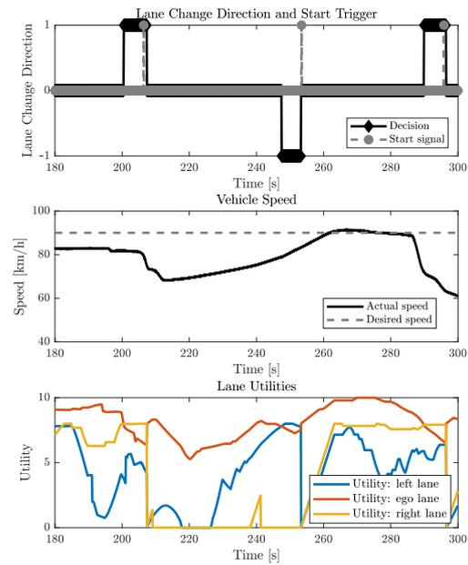
Figure 4: Lane change decisions, Lane utilities and vehicle speed during a part of autonomous driving.
