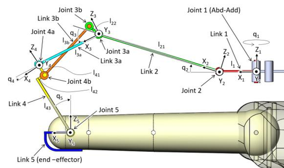
Figure 9: Kinematic model of the robots. A frame  $R_i=(O_i, X_i, Y_i, Z_i)$  is associated with each link, with its origin positioned on the joint axis,  $q_i$  is the rotation around joint  $i$ , and  $l_i$  (resp.  $l_{i1}, l_{i2}$ ) designates the length of link  $i$  (resp. of different parts of link  $i$ ).
