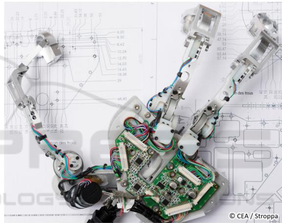
Figure 13: Internal view of the manufactured prototype of tri-digital dexterous hand master.
