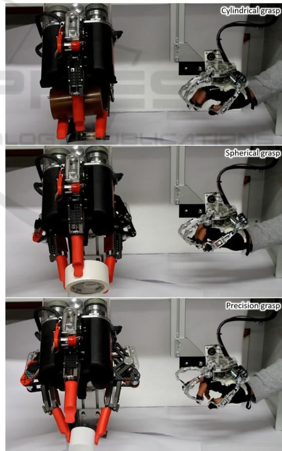
Figure 17: Dexterous teleoperation with force feedback using the tri-digital hand master.
