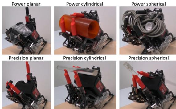
Figure 2: Illustration of the possible grasps of the CEA LIST's three fingers slave hand.
