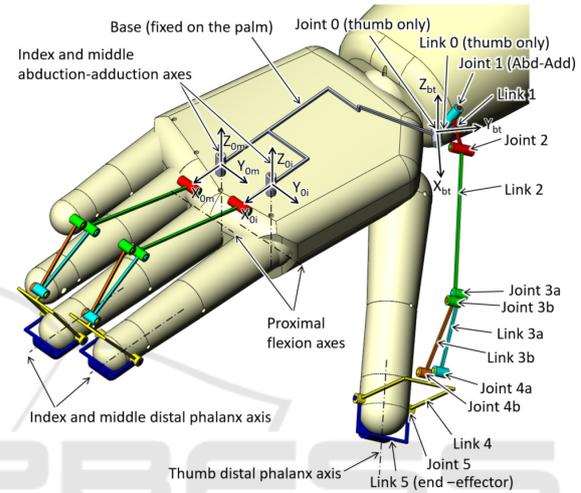
Figure 8: Kinematic model of the master glove ( $R_{bt}(O_{bt}, X_{bt}, Y_{bt}, Z_{bt})$ , resp.  $R_{oi}=(O_{oi}, X_{oi}, Y_{oi}, Z_{oi})$  and  $R_{om}=(O_{om}, X_{om}, Y_{om}, Z_{om})$  are the base frames of the thumb, index and middle fingers).
