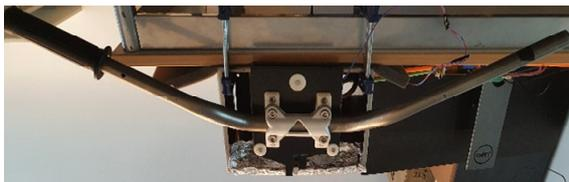
Figure 3: Haptic feedback motorcycle handlebars used in our POC system.
