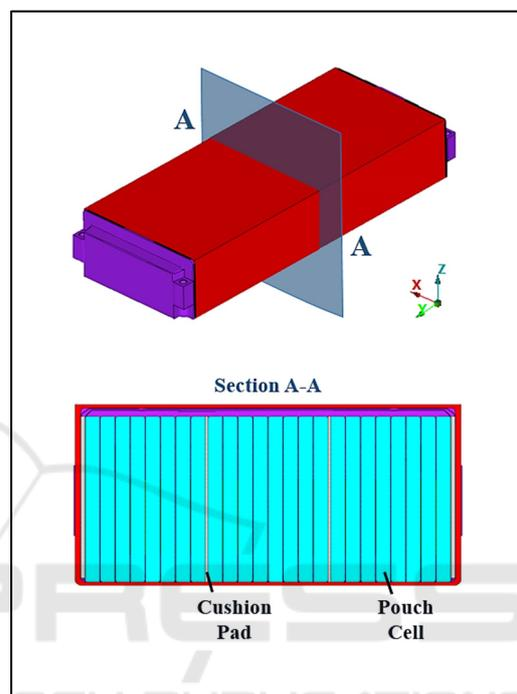
Figure 2: CAD-model of the examined battery module.
