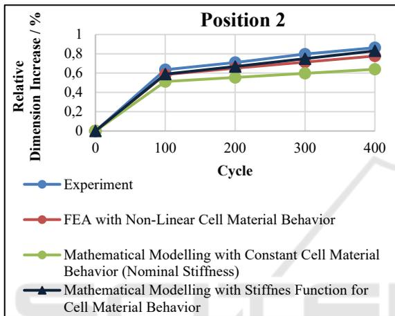
Figure 8: Comparison of battery module relative dimension increase in experiment and simulation at position 2.
