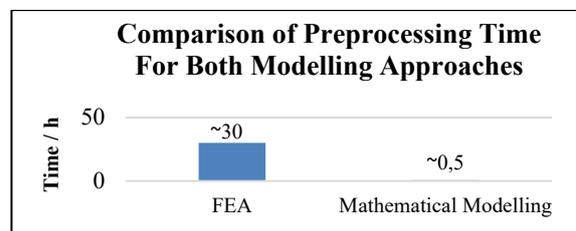
Figure 4: Comparison of preprocessing time for both modelling approaches.
