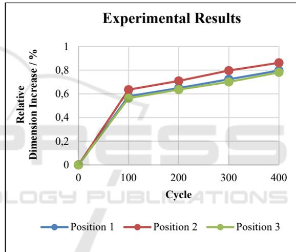
Figure 7: Experimental results for battery module swelling.
