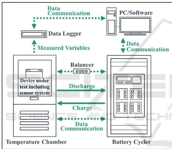
Figure 5: Experimental setup for deformation measurement of battery modules.
