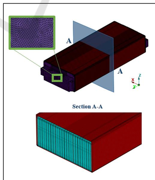
Figure 3: Meshed model of the examined battery module.
