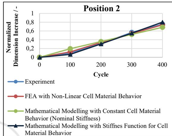
Figure 10: Comparison of battery module normalized dimension increase in experiment and simulation at position 2.
