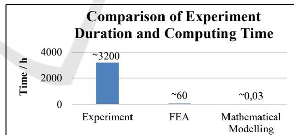
Figure 11: Comparison of computing time and experiment duration.
