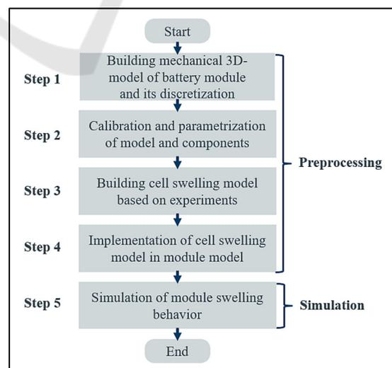
Figure 1: Schematic representation of the simulation method for swelling prediction of battery modules.
