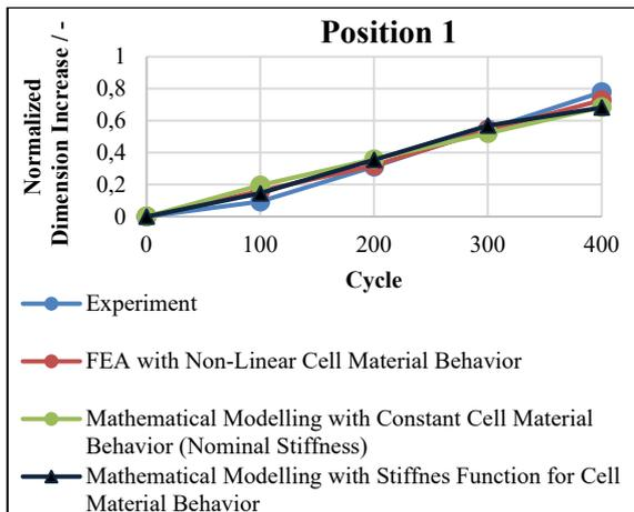
Figure 9: Comparison of battery module normalized dimension increase in experiment and simulation at position 1.
