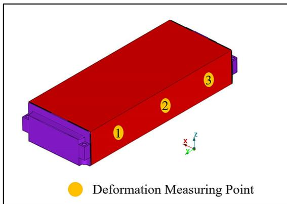
Figure 6: Swelling measurement points on device under test.
