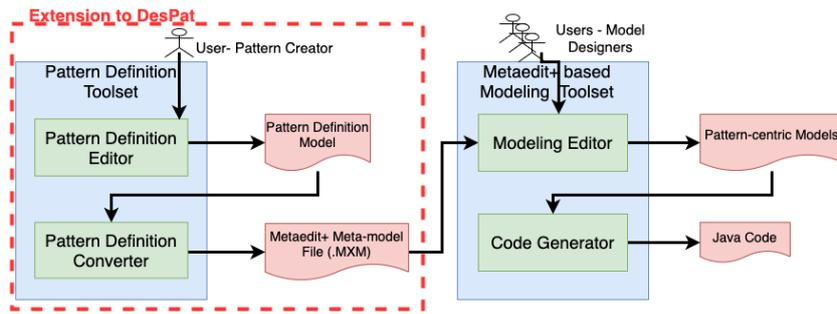
Figure 3: *DesPat*'s extended tool architecture.
