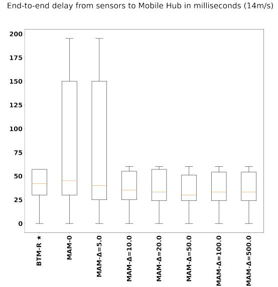
Figure 1: Average delay comparison between BTM-R and MAM relay with least-hop route.
