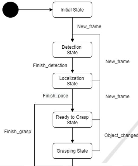
Figure 3: State machine of the pose estimation module.
