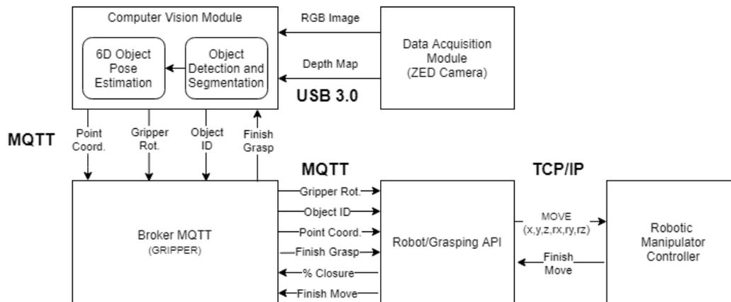
Figure 1: General system architecture with data flow illustration.
