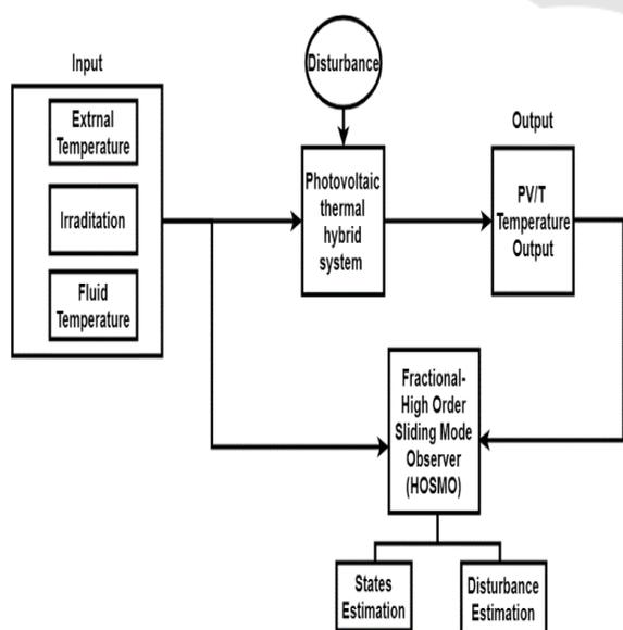
Figure 1: Disturbance & States estimation of the system.
