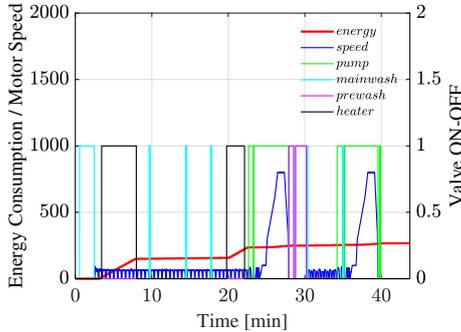
Figure 3: Input-output data for the QUICKWASH program.
