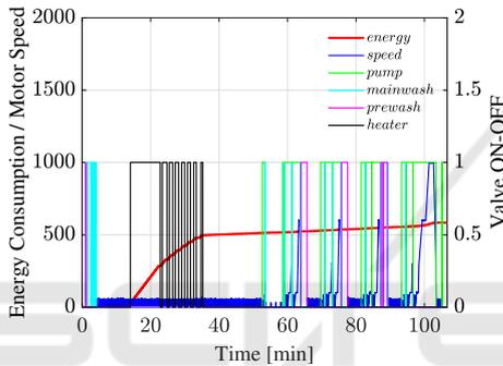
Figure 4: Input-output data for the BEDDING program.
