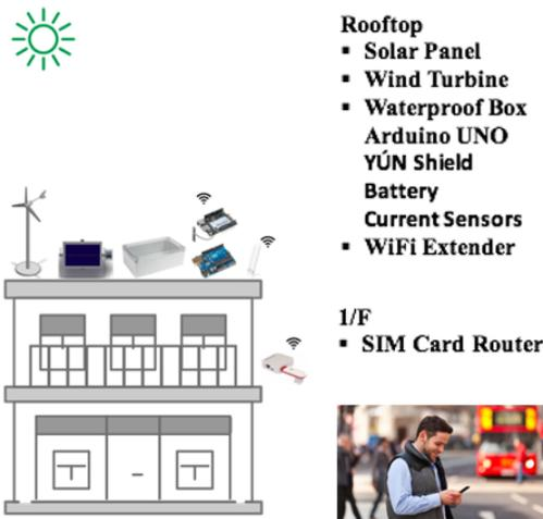
Figure 2: Proposed residential installation of the system.
