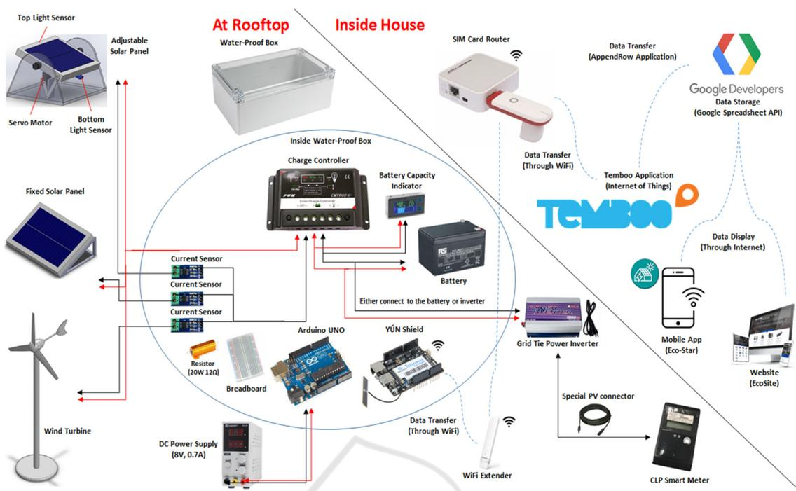
Figure 1: The schematic diagram of the smart IoT system for monitoring and enhancing renewable energy feed-in tariff at household or small office in Hong Kong or similar developed cities.
