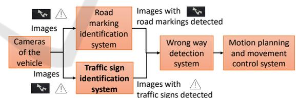
Figure 1: Example of a wrong way detection system of an automated vehicle, which uses inputs from traffic sign detection system and road marking detection system.
