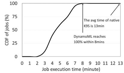
Figure 8: The distribution of the training job execution time under DynamoML.
