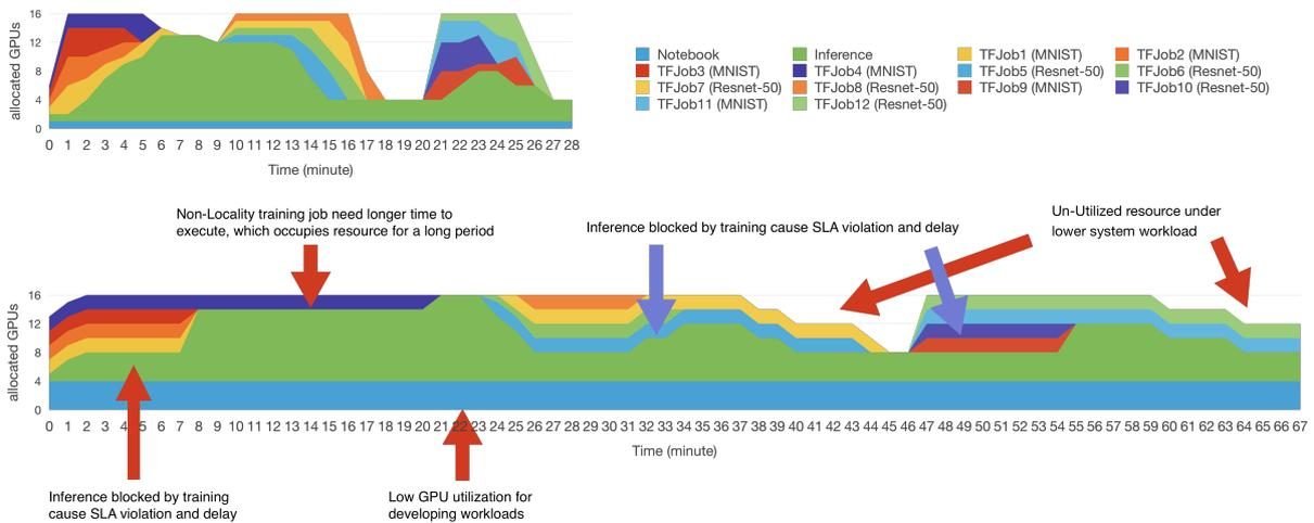
Figure 5: The overall resource allocation for DynamoML (top) and K8S+Scaling (bottom).
