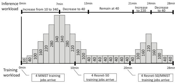
Figure 4: Testing workload for system evaluations. The workload of interface jobs are time-varied by adjusting the number of active users. The workload of training jobs are submitted in 4 groups and 4 jobs per group at time 0, 10, 20. The modeling jobs are consisted of 4 notebook instances persistently running throughout the experiments.
