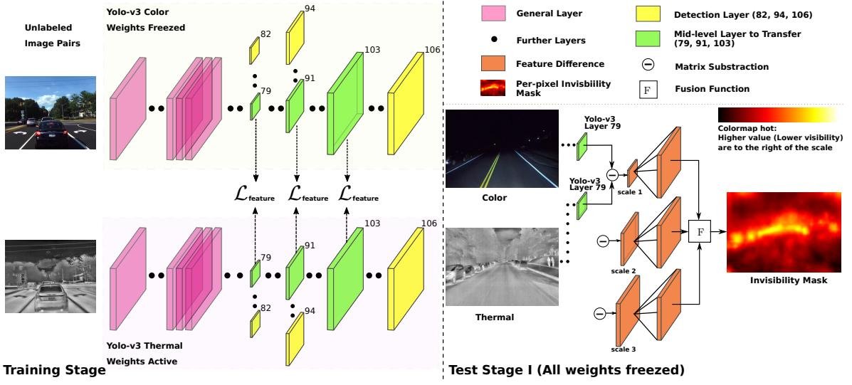
Figure 2: System overview. Our system takes well-aligned image pairs from unlabeled video streams. In the training stage (left), the Yolo-v3 color network is frozen, while Yolov3-thermal network is trained to reproduce the mid-level features as the ones in Yolov3 color network at three scales in layer 79, 91 and 103 of the network. In the test stage (right), the difference of those features from layer 79, 91 and 103 are computed and fused to get the final invisibility mask.
