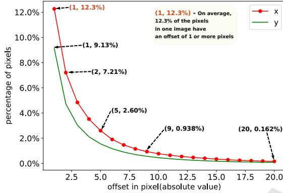
Figure 6: X-Y offset distribution. We show that in the image plane offset in x direction is on average larger than that in y direction. Also distinct movements(5 pixels or more) constitute 2.6% of the pixels in the images.
