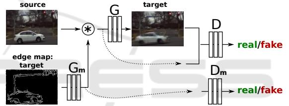
Figure 3: Base alignment network. The module takes as input source image and edge map from target position, and outputs the target image in the given position. The conversion from source to target, performed using network  $G$  is conditioned on the motion cues generated using network  $G_m$ . The target prediction after network  $G$  and motion cues generated by  $G_m$  are fed into two discriminators  $D$  and  $D_m$  respectively.
