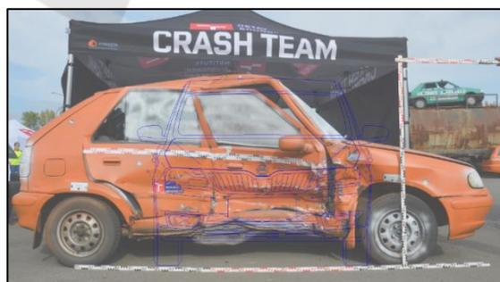
Figure 2: Damage correspondence - crash test 1.
