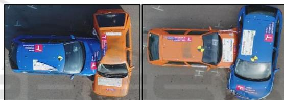
Figure 1: Crash tests configuration.
