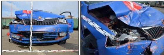
Figure 3: Vehicle Skoda Rapid after crash test 1.
