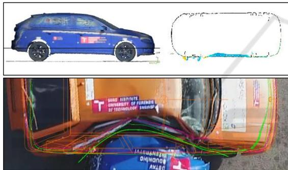
Figure 9: The measurement of deformation depth using 3D scanner.
