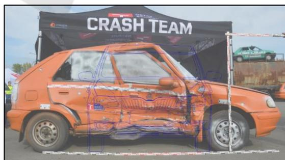
Figure 2: Damage correspondence - crash test 1.
