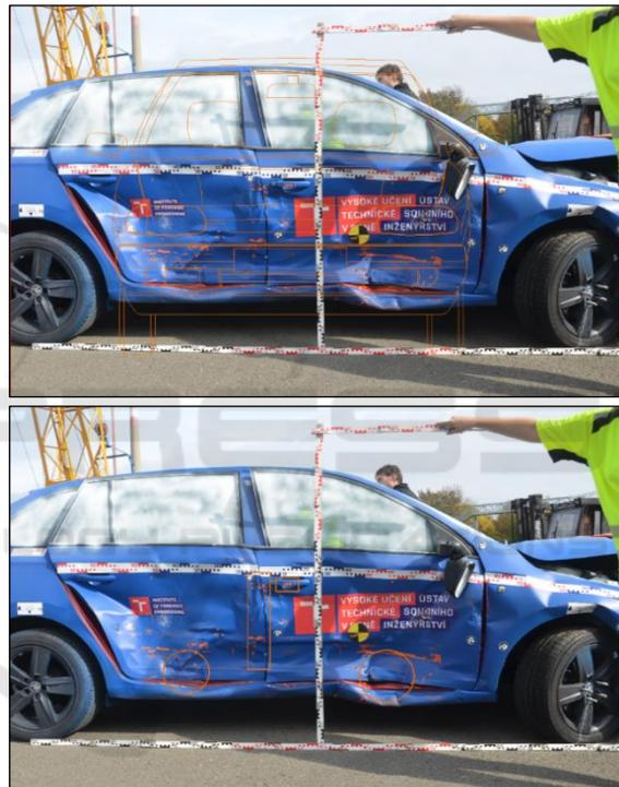
Figure 6: Vehicle Skoda Rapid after crash test 2.
