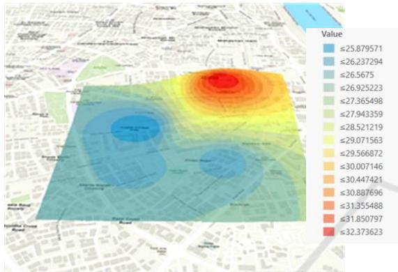
Figure 9: Occupancy at Paldi junction in April 2019 20:00 (value shows the level of occupancy).
