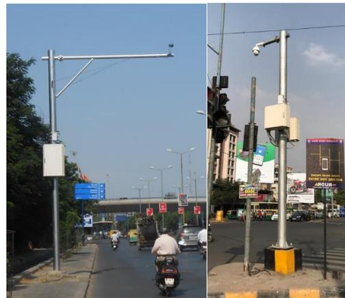
Figure 4: Traffic monitoring camera (left picture) and Surveillance camera (right picture).
