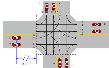
Figure 3: Geometry of the 16-lanes intersection.
