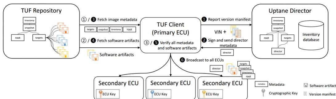
Figure 3: TUF+Uptane Architecture (Asokan et al., 2018).
