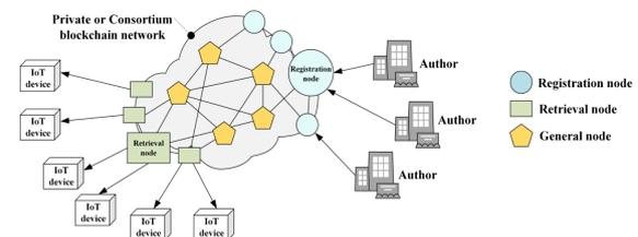
Figure 5: Blockchain-based firmware update platform (Lee and Lee, 2017).
