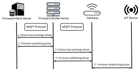
Figure 2: MQTT-based design.
