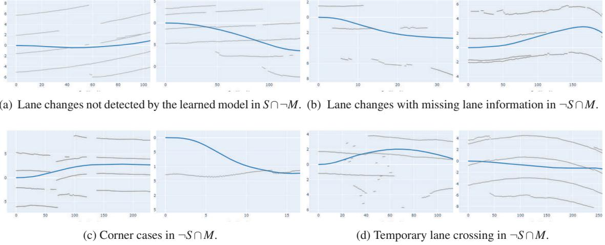
Figure 5: Lane changes where the improved labels  $M_l^r$  and detections  $S_l^r$  from the corresponding learned model do not match. Also corner cases with modified lanes due to roadwork or holding on the sidewalk where found (c).
