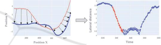
Figure 6: Trajectories from the ego vehicle in blue and a detected object in red (left). The decreasing minimal distance between the trajectories is used for cut-in detection (right).
