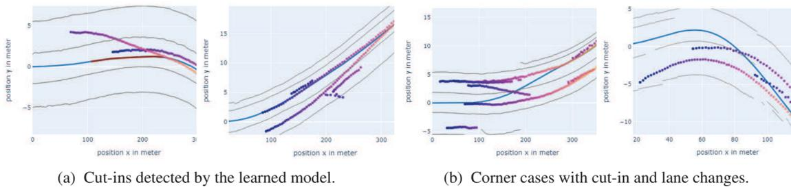
Figure 8: Top-Down visualization of not labeled cut-ins detected by the learned model ( $\neg S \cap M$ ). The ego trajectory is shown in blue, detected lane markings in grey and the trajectories of detected objects are color encoded with brighter colors with ongoing time.
