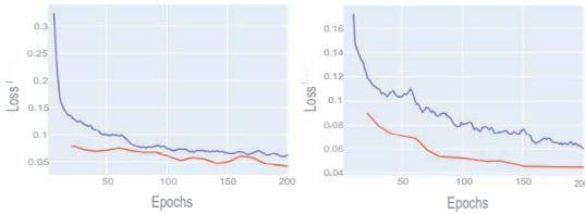
Figure 4: Training loss (blue) and validation loss (red) for two models trained with labels from the simple rule-based detector (left) and the improved rule-based detector (right).
