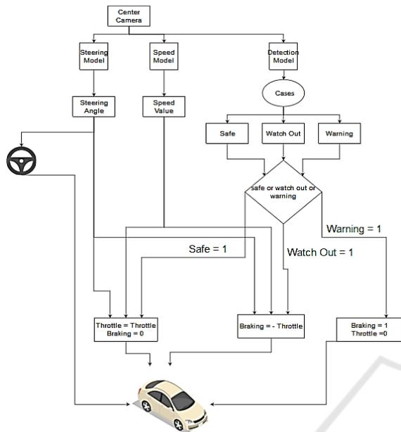
Figure 2.1: Processes implemented to control autonomous car flowchart.
