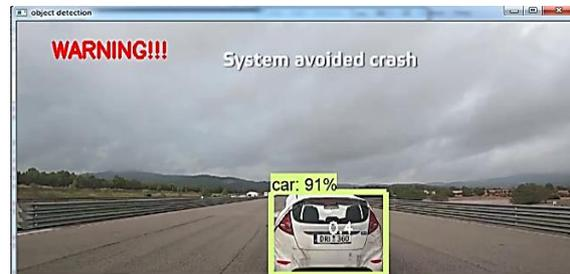
Figure 3.2: Second warning displayed when there is a close car.
