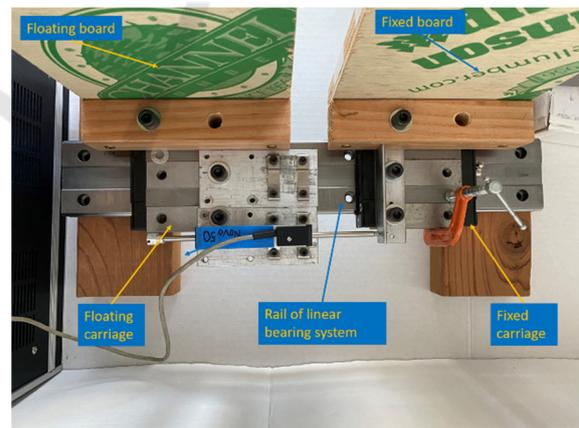
Figure 3: Top view of experimental setup: linear bearing system with carriages.
