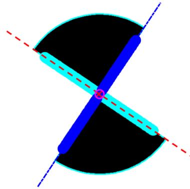
Figure 9: Step 2: Target's center as intersection of two straight lines best fit to the transition points.
