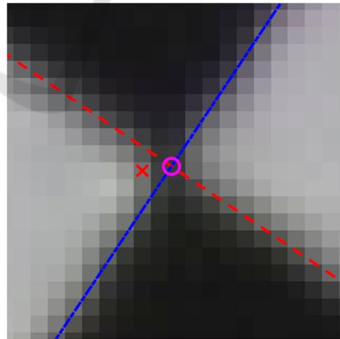
Figure 10: Target's center: step 1 (red cross) and step 2 (magenta circle).
