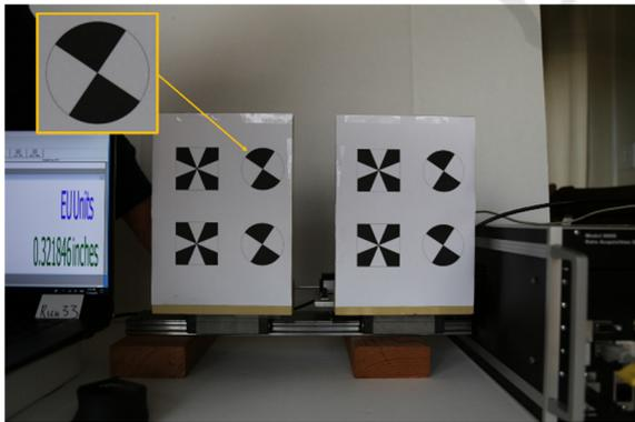
Figure 8: Step 1: find target's pattern in image.
