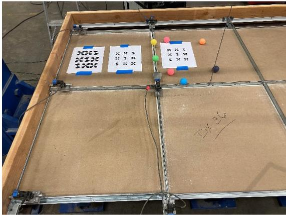
Figure 1: Monitoring grid and panel displacements in testing of suspended ceiling system.
