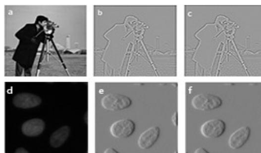
Figure 8: A: the original image, b: image filtered in MATLAB and c: FPGA generated image with Laplacian filter; d: original nucleus image, e: MATLAB generated image and f: the FPGA generated image with median and first derivative filter.
