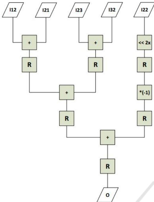
Figure 3: Pipeline adder tree.
