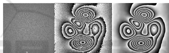
Figure 4: (a) noisy fringe pattern; (b) noisy extracted phase using the Fourier transform method; (c) denoised phase using WFT.
