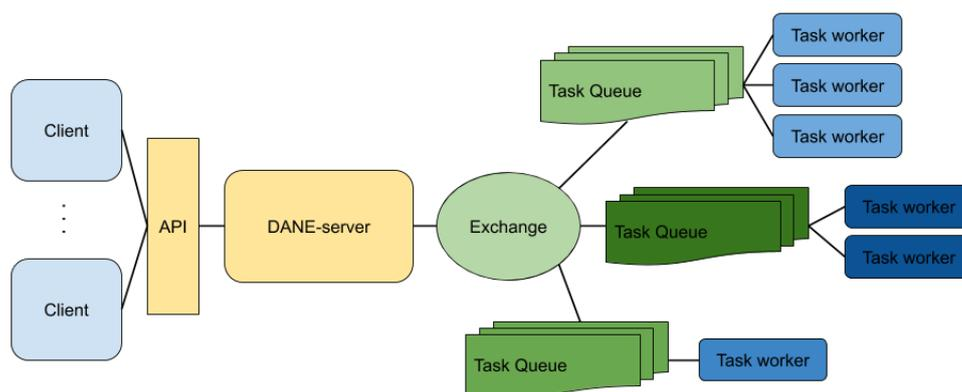
Figure 2: Schematic overview of the DANE architecture that illustrates the components that mediate the interaction between clients (the consumers of the results), and the workers (the producers of the results).
