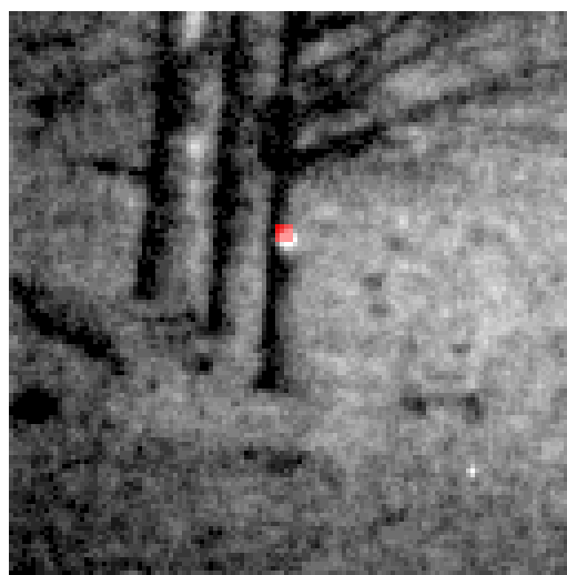
Figure 7: B/W image of the outdoor scene at 128 \times 128 pixel resolution, reconstructed using a subsampling ratio of 18%. The \varnothing 7 cm reflector, seen as a bright dot when the laser is continuously on, is mounted on a tree at 350 m range. The red overlaid image of the simulated 1 ms light flash is reconstructed to 32 \times 32 pixel resolution using 20 consecutive patterns (during a pulse) and illustrates the capability to detect and localize the flash at the same position as the reflector (ground-truth).
