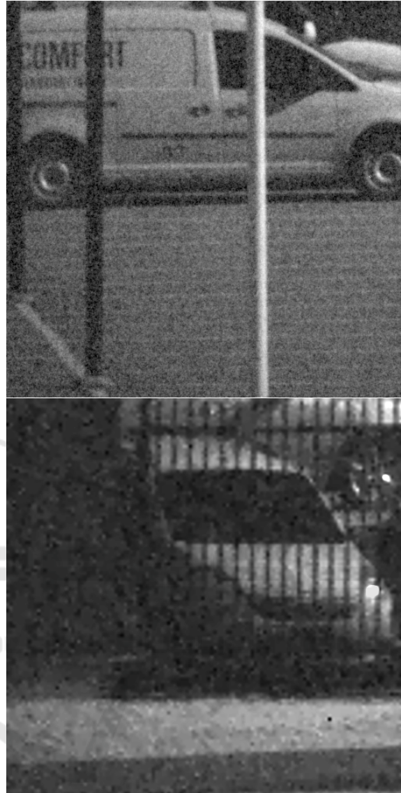
Figure 4: Two images of cars at 512x512 (top) and 256x256 (bottom) pixel resolutions at 350 m. Subsampling ratios are 30% and 40%, respectively. In the bottom image a fence can be seen in the foreground (seen as thin horizontal lines).
