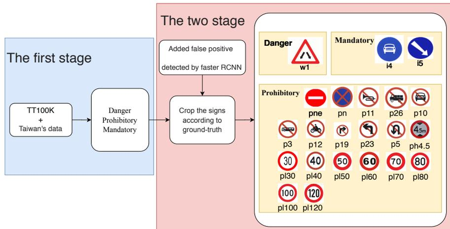
Figure 5: The two-stage processing flowchart with three-category detection. The network training of the first stage is for all signs or three categories. In the second stage, the background false positives are added for training.
