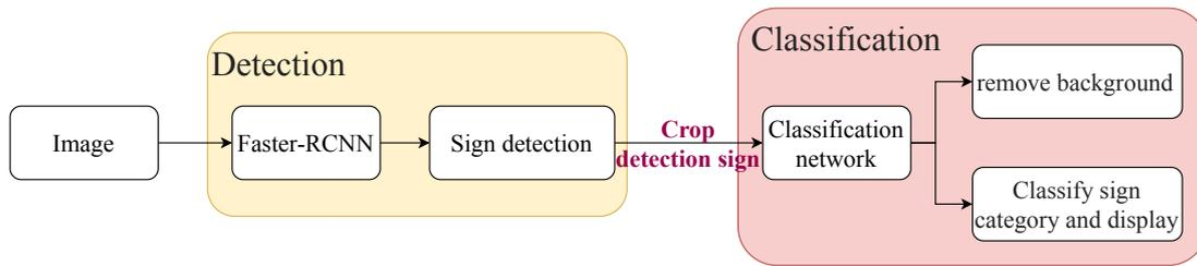
Figure 1: The flowchart of the proposed two-stage traffic sign detection and recognition.
