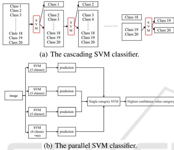
Figure 2: Two different SVM variations (cascading and parallel) used for the second stage.
